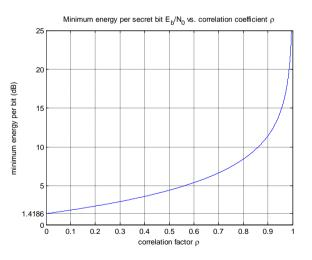
Fig.3Minimum energy per secret bit  $E_b/N_{0 \text{ min}}$ , vs. Correlation coefficient  $\rho$ .
