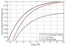
Fig .4 Secrecy capacity in bits/s/Hz/dimension vs. energy per secret bit  $E_b/N_{0 s}$  when  $n_T$ = 1,  $n_R$ = 5, and  $n_E$ = 3.
